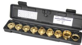
Used for router template following on template patterns or jigs. Set includes 8 bushes to suit router bases with a 30mm hole. Outside diameters include: 5/16", 3/8", 7/16", 1/2", 39/64", 13/16", 1" and 1-3/8". Locking nut included.
