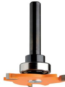
Use the CMT slot cutter to rout grooves, rebates and T-slots; or the relief to start dovetail joints on wood panels. Each bit features three carbide-tipped cutters, orange coloured PTFE coating and anti-kickback design. The 22mm (7/8") bearing is included for a cutting depth of 12.7mm (1/2"). The bit and the slot cutter are also available separately.
